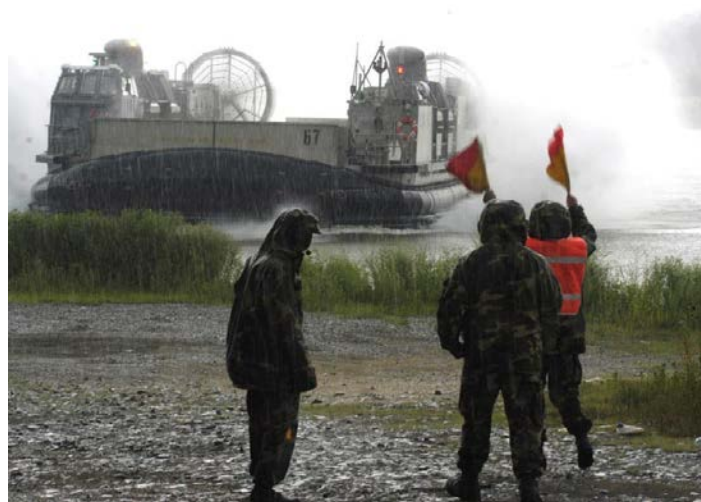
CBIRF uses a Landing Craft Air Cushioned (LCAC) vessel to validate water routes along the Potomac River. The hovercraft is nearly 90 feet long, can lift more than 60 tons of cargo, and is capable of speeds in excess of 40 knots. (U.S. Navy photo)
