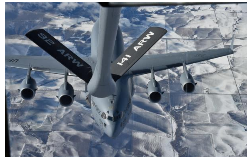
Image: A KC-135 Stratotanker from Fairchild Air Force Base refuels a C-17 Globemaster III from JBLM during a training flight over Eastern Washington. Credit: 92nd Air Refueling Wing Public Affairs, M. Mendez, 2016, dvidshub.net
